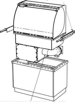
FLEXIBLE DUCTING & IN-LINE FAN SUPPLIED LOOSE. RE-ATTACH FLEXIBLE DUCTING & IN-LINE FAN TO SIDE OF COMPRESSOR CRADLE ONCE UNIT HAS BEEN DROPPED INTO PLACE. ELECTRICALY CONNECT FAN TO CONTROL BOX WITH "KETTLE PLUG"
