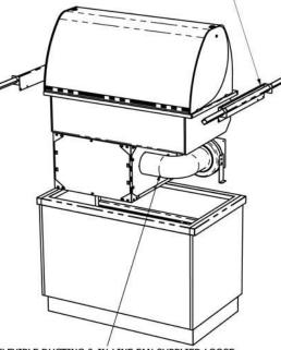
FLEXIBLE DUCTING & IN-LINE FAN SUPPLIËD LOOSE. RE-ATTACH FLEXIBLE DUCTING & IN-LINE FAN TO SIDE OF COMPRESSOR CRADLE ONCE UNIT HAS BEEN DROPPED INTO PLACE. ELECTRICALY CONNECT FAN TO CONTROL BOX WITH "KETTLE PLUG"
