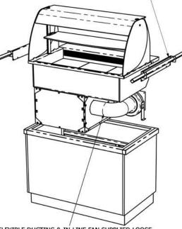
FLEXIBLE DUCTING & IN-LINE FAN SUPPLIED LOOSE. RE-ATTACH FLEXIBLE DUCTING & IN-LINE FAN TO SIDE OF COMPRESSOR CRADLE ONCE UNIT HAS BEEN DROPPED INTO PLACE. ELECTRICALY CONNECT FAN TO CONTROL BOX WITH "KETTLE PLUG"
