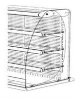
LOCATE SHELF SUPPORT BRACKETS INTO REAR SLOTS AT HEIGHT & ANGLE TO SUIT PRODUCTS. PUSH ON 3 x GREY SILICON SHELF RESTS ONTO EACH BRACKET BEFORE GLASS SHELVES ARE LOWERED ON.
