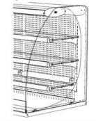
LOCATE SHELF SUPPORT BRACKETS INTO REAR SLOTS AT HEIGHT & ANGLE TO SUIT PRODUCTS (NOTE: 2 No. BRACKETS WITH GLASS STOPS TO BE FITTED AT BTM.). PUSH ON 3 x GREY SILICON SHELF RESTS ONTO EACH BRACKET BEFORE GLASS SHELVES ARE LOWERED ON (NOTE: 1 No. SHORT SHELF TO BE FITTED AT BTM.)
