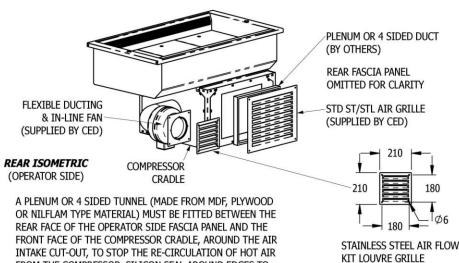
INTAKE CUT-OUT, TO STOP THE RE-CIRCULATION OF HOT AIR FROM THE COMPRESSOR. SILICON SEAL AROUND EDGES TO ENSURE THERE ARE NO AIR GAPS.
