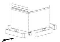
NOTE: KICKPLINTH SUPPLIED AS STANDARD IS SUITABLE FOR LOWEST ADJUSTED UNIT HEIGHT
