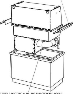
FLEXIBLE DUCTING & IN-LINE FAN SUPPLIED LOOSE. RE-ATTACH FLEXIBLE DUCTING & IN-LINE FAN TO SIDE OF COMPRESSOR CRADLE ONCE UNIT HAS BEEN DROPPED INTO PLACE. ELECTRICALY CONNECT FAN TO CONTROL BOX WITH "KETTLE PLUG"
