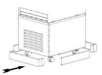
NOTE: KICKPLINTH SUPPLIED AS STANDARD IS SUITABLE FOR LOWEST ADJUSTED UNIT HEIGHT
