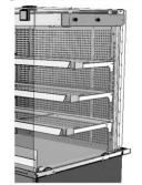
LOCATE SHELF SUPPORT BRACKETS INTO REAR SLOTS AT HEIGHT & ANGLE TO SUIT PRODUCTS (NOTE: SHORTEST BRACKETS AT TOP AND LONGEST BRACKETS AT BTM). REST GLASS SHELVES ONTO RUBBER BUMPERS ON SHELF SUPPORTS. (NOTE HALF-LENGTH SHELVES ARE LOCATED ON BOTTOM TO ALLOW FOR TALLER BOTTLES ON DECK)
