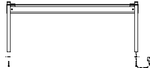
2 x FIXING/SPREADER PLATES (SUPPLIED) 4 x M8 FIXING BOLTS (SUPPLIED)
